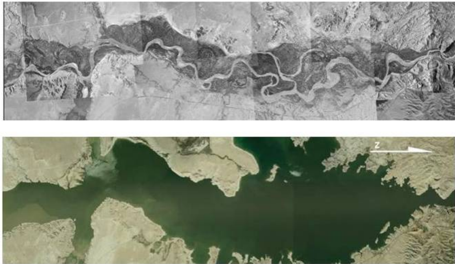
Fig 3: Aerial imagery of the Wind River before and after the inundation of Boysen Reservoir (1948 and 1949 georeferenced photo mosaic and 2006 orthophotos, USGS)
